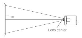
The projector lens should be centered in the middle of the screen.
